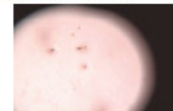
Post-process using Slurry 2 - Post CMP Roughness = 121A Ra, Removal Rate = 4.0 \mu\text{A}/\text{min} . Surface showing some improvement, heavy pitting caused by the slurry.
